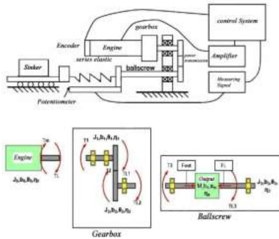
Figure 2: Series elastic mechanism
