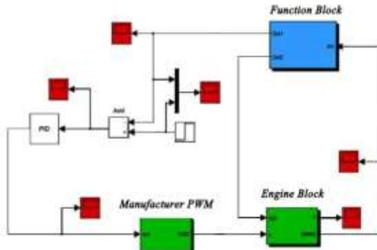
Figure5: General model system controller
